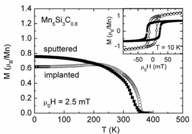
**Figure 2.** Magnetization  $M(T)$  of magnetron sputtered (closed symbols) and  $\text{C}^+$ -ion implanted (open circles)  $\text{Mn}_5\text{Si}_3\text{C}_{0.8}$  films. Insets show  $M(H)$  loops taken at  $T = 10 \text{ K}$ .
