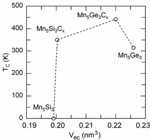
**Figure 3.** Curie temperatures of  $Mn_5Si_3$  (antiferromagnetic,  $T_C = 0$ ),  $Mn_5Si_3C_{0.8}$ ,  $Mn_5Ge_3C_{0.8}$ , and  $Mn_5Ge_3$  vs volume of the hexagonal unit-cell.
